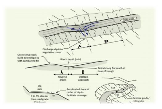
percent and require that any outside berm be removed for the entire length of the rolling dip. The outlet of the rolling dip shall be protected with rock, logs, branches, or brush to minimize erosion.
