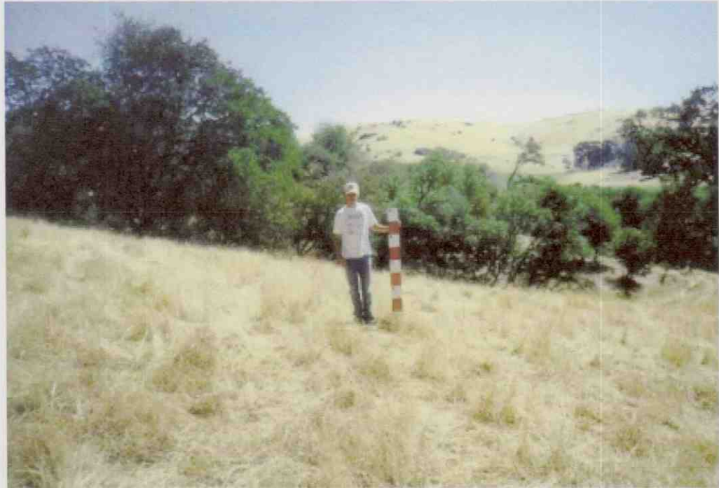
Figure 7. You can use a profile board to indicate scale in a photograph.
