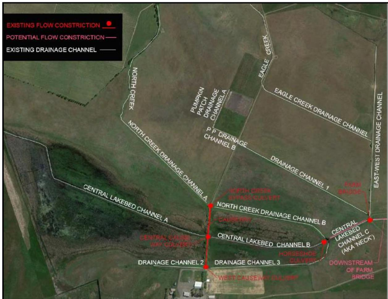
**Figure 4.** Existing Irrigation Channels and Hydraulic Structures in Tolay Lake Regional Park (WRA 2013).
