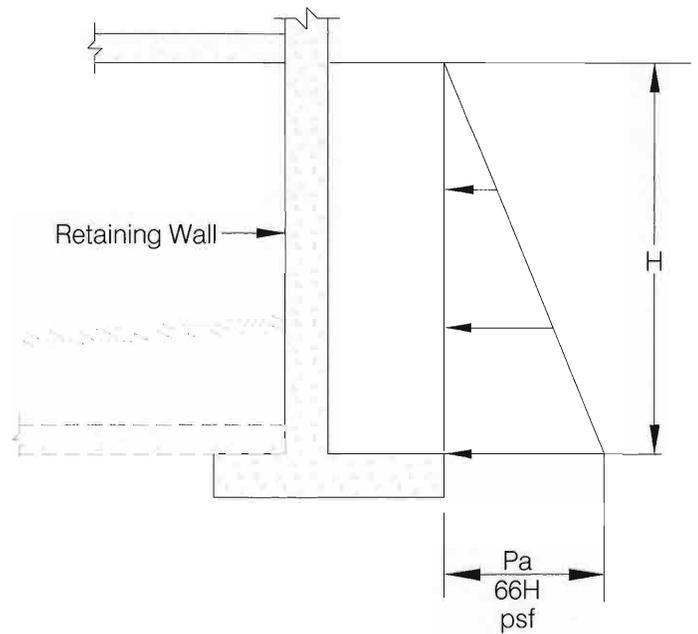
**AT-REST SOIL PRESSURES DIAGRAM**
