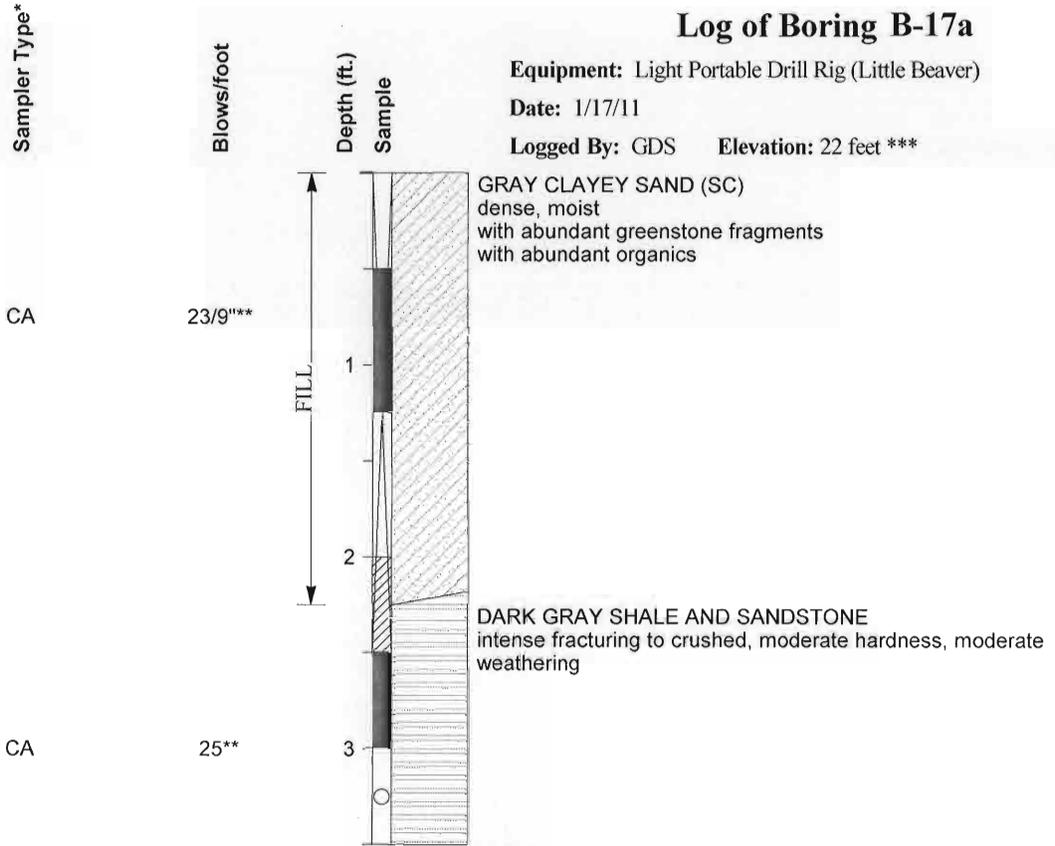
\*CA - California Modified Split Barrel Sampler 3.0-inch O.D.
