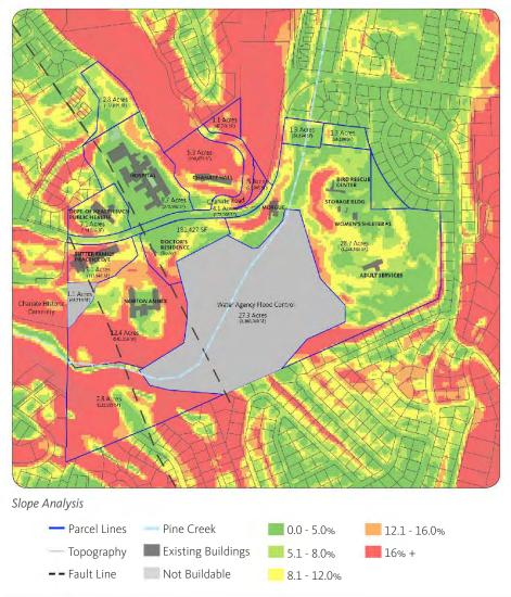
The Chanate site poses a challenge to development due to its rugged topography. Much of the site is sloped to varying degrees and would require a "cut and fill" approach to creating buildable lots. The map at right identifies the different categories of slope.
