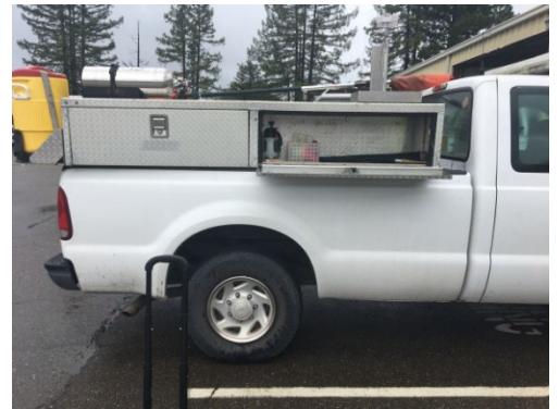
Utility Bed on Pick-up Bottom of Storage at 55" from ground- Storage for Herbicide or chainsaws
