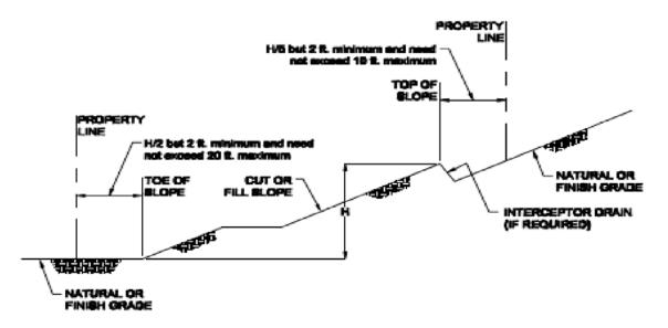
Figure 11-2 Cut and Fill Slope Setback Requirements
