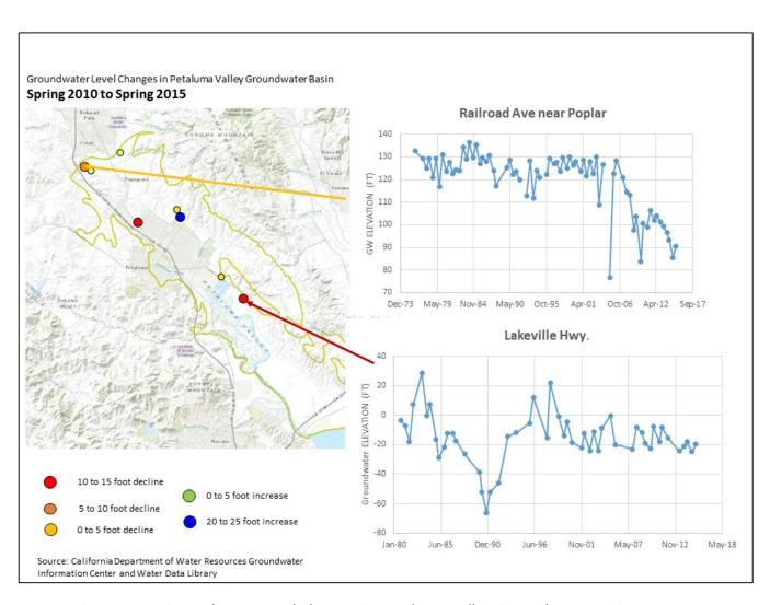
Figure PV-1. Groundwater Level Changes in Petaluma Valley Groundwater Basin
