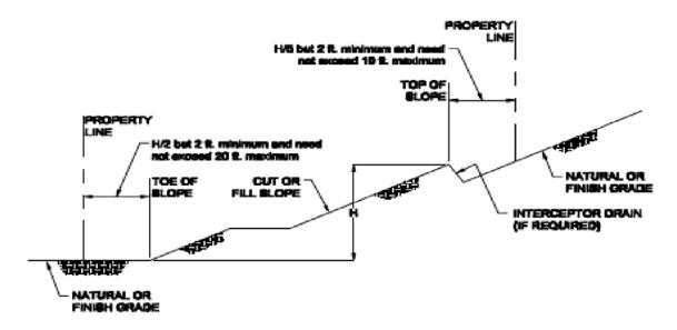
Figure 11-236-2 Cut and Fill Slope Setback Requirements
